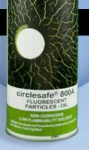
CircleSafe® 800A is an aerosol spray can of Mi-Glow® 800 fluorescent yellow-green particles and CircleSol M<sup>™</sup>, a refined petroleum distillate. It is designed to detect very fine discontinuities found in finished products and critical, highly stressed component parts. Its ultra-bright, ultra-sensitive particles allow for excellent detection. The carbon dioxide propellant reduces combustible hazard.
